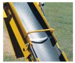
Enhance efficiency. The unit's side-discharge conveyor belt allows operators to load processed material into dumpsters or pickup trucks, or to create windrows of processed material.
