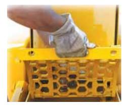
Save time with one-person screen change. Operators can load screens by hand without the use of additional support equipment or personnel.
