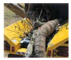
Increase grinding productivity. The patented Vermeer SmartFeed system monitors engine rpm rates and automatically stops and / or reverses the feed roller and feed conveyor to help enhance production.
