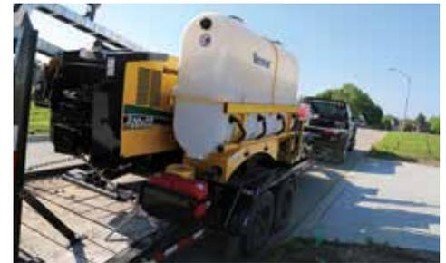
**NARROW WHEN YOU NEED IT.** The D20x22 S3 features a shorter, narrower design and is lighter weight than comparative competitive models, which allows for it to sit comfortably on a trailer when paired with a mix system.
