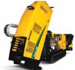
**SERVICEABILITY.** The drill's flip-up metal hood offers ease of access when performing routine service and maintenance.
