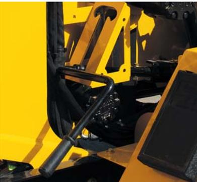
**A clutchless PTO system** reduces premature wear to the belt-drive system by preventing high-speed engagement of the cutter drum. The throttle is integrated with the belt drive to help ensure the PTO can be engaged only while the engine is at low speed.
