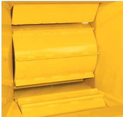
**Dual horizontal offset feed rollers** improve performance by aggressively grabbing and feeding material to the drum. The offset helps the upper feed roller climb over big logs or material with lots of branches or forks.
