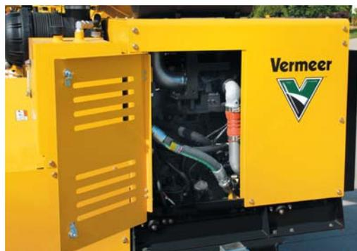
**Engine options to fit your needs.** With two Cummins diesel engine options providing 85 hp (63.4 kW) or 110 hp (82 kW), contractors have the ability to choose an appropriate horsepower option based on their jobsite. A steel engine enclosure helps provide additional durability.
