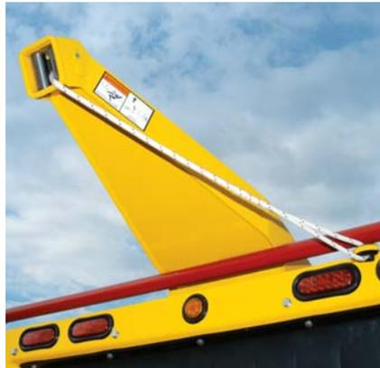
**Easily lifts heavy material.** An optional winch allows operators to move large logs effortlessly. The 150' (45.7 m) winch line can handle logs up to 2000 lb (907.2 kg) and can be used to lift the log onto the feed table.
