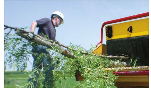
**SMARTFEED.** The patented SmartFeed system helps increase operator productivity while reducing strain on vital engine parts. The feed-sensing control system monitors engine rpm and automatically stops and reverses the feed roller when feeding larger, hardwood material.
