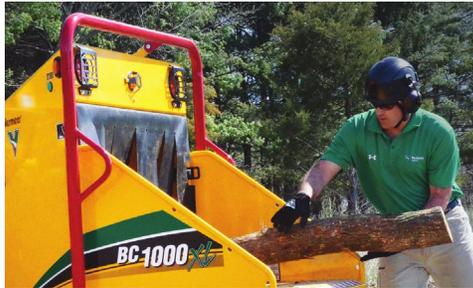
**OPERATOR SAFETY.** Combined with the patented Bottom Feed Stop Bar is the four-position upper feed control bar with dual stop positions and forward/reverse feed positions. Mounted over the feed table, it enables the operator to stop the feed rollers and select forward or reverse operations. Dual reset/hold-to-run buttons allow the operator to readily reset the Bottom Feed Stop Bar.
